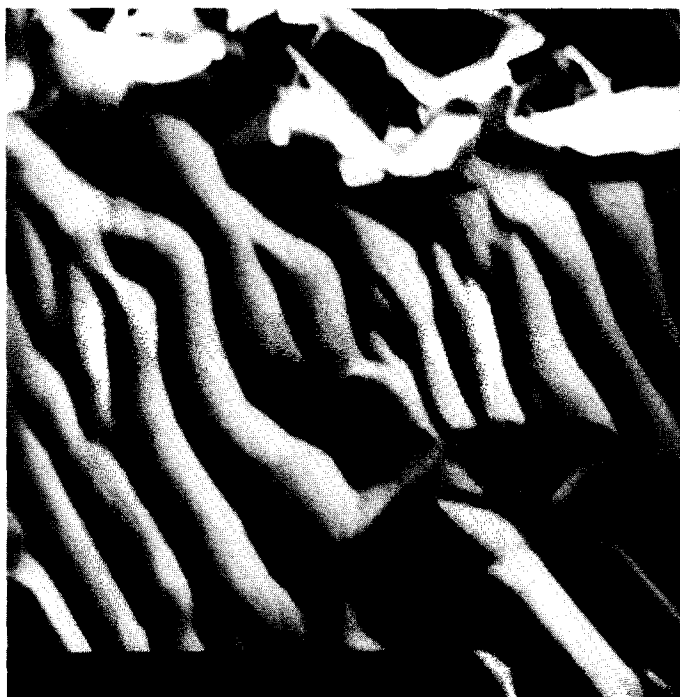
FIG. 8. Scanning electron micrograph of the sample coated with a thin layer of Mg after 100 hr of operation \times 1000 .
