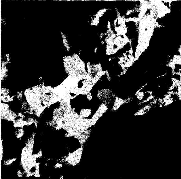
FIG. 7. Scanning electron micrograph of the standard sample after 300 hr of operation \times 1000 .
